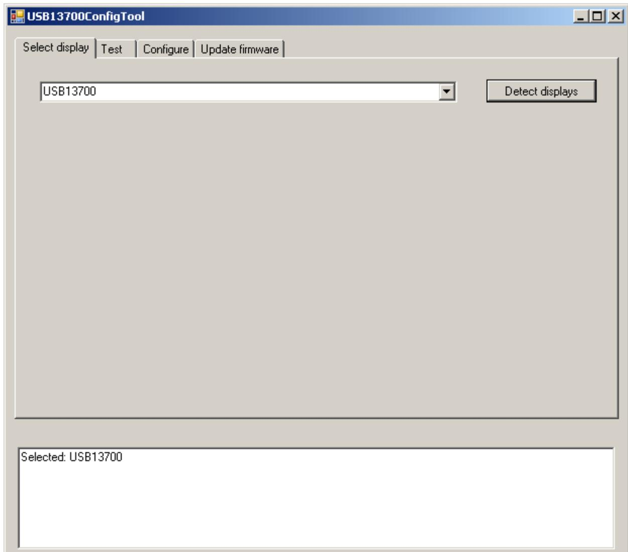
In the Test tab you can do some simple testing. Pressing the 'Test' button shows 5 horizontal lines on the display. Two lines to the top of the display, two lines to the bottom and one line in the middle.
